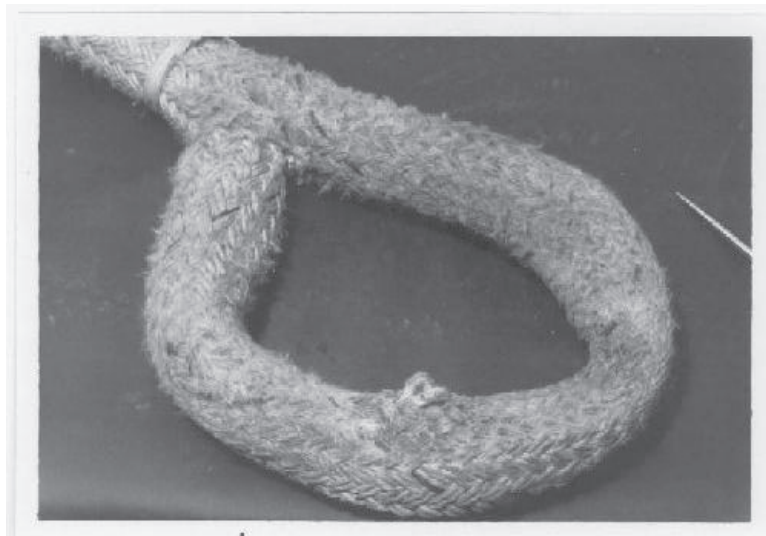
Figure D-019 Wear in Double Braid Eye Splice
