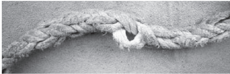
Figure D-004 Matted Internal Yarns (Exposed strands reveal internal matting)
