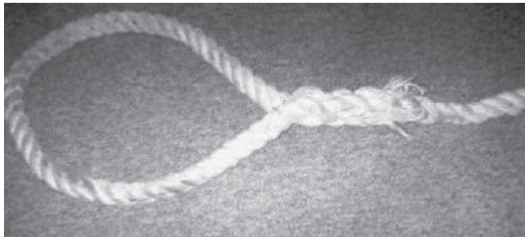
Figure D-018 3-Strand Splice of Poor Quality
