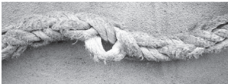
Figure D-013 Pulled Strand in 8 Strand Rope
